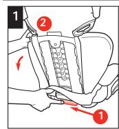
To remove backrest from seat base, backrest needs to be in the most upright position. Press down firmly on backrest release tab and rotate seat back until it lays flat.
